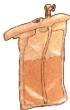
The In-Suit Drinking Device (ISDD) for use on Apollo 14-17 holds up to 32 ounces of drinkable water.
